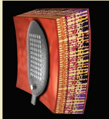
FIGURE 8 This light-sensitive chip is implanted into the eye's retina and is able to convey visual information into ganglion cells and ultimately to the brain. (Source: Adapted, with permission, of IEEE Engineering and Medicine and Biology 25:15 (2005).)
