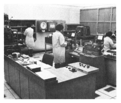
**Figure 12** A precision measurement center is a precisely controlled environment for highaccuracy calibration of gage blocks, master rings, disks, and other precise measurement applications.
