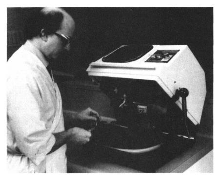
Figure 7 Abrasive cutter used to section rigid materials.
