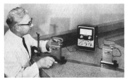
Figure 17 Electronic levels in surface plate calibration setup. (Courtesy of Federal Products Corporation.)
