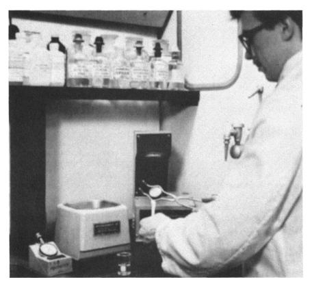
Figure 14 Etching a metallographic sample.
