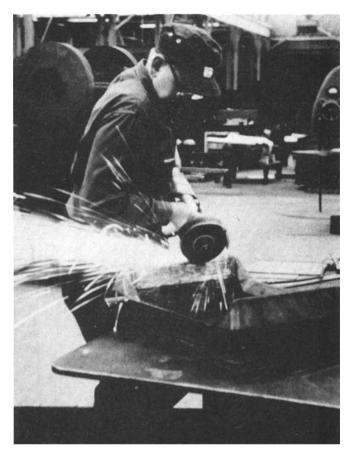
Figure 2 Snagging operation using an offhand grinding machine.
