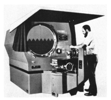
**Figure 4** An optical comparator inspects the threaded portion of a splined shaft. The system features a 30-in. screen plus digital readout of the horizontal and vertical position of the part. The machine can be interfaced with instrumentation such as computers, printers, a vector positioner, and so on. (Courtesy of Jones & Lamson Metrology Systems, Waterbury Farrel Division of Textron, Inc.)
