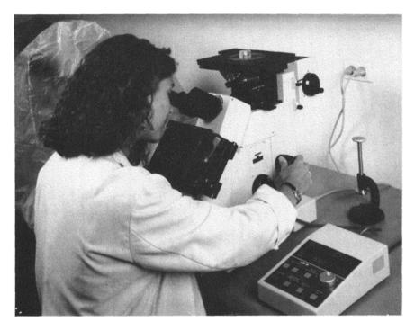
**Figure 15** An inverted-stage metallograph used to examine, analyze, and photograph the microstructure of materials from polished specimens.
