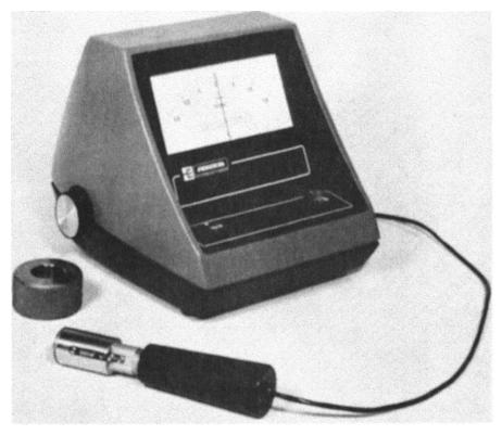
**Figure 9** Fast, reliable bore measurement is possible with electronic plugs. (Courtesy of Federal Products Corporation.)
