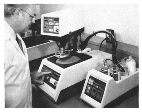
**Figure 13** An automatic grinder/polisher used to prepare larger quantities of uniformly polished specimens for metallographic examination.
