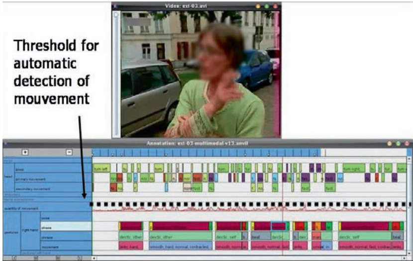
Fig. 15.1 Integration in the Anvil tool (Kipp, 2004) of manual annotations (colored blocks) of head movements (upper tracks) and hand gestures (lower tracks), and results of image processing for the estimation of movement quantity (continuous line in the middle)
