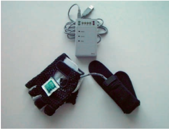
Fig. 16.3 In EREC-II, the sensing circuitry is accommodated by a wrist pocket, making the glove lighter and more airy. It also allows for more flexible system arrangements.
