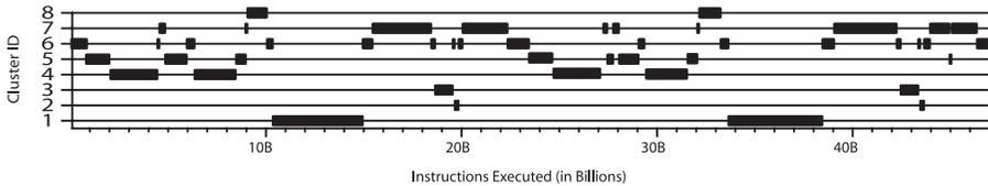
**Figure 7.6** Shows which intervals during the program’s execution are partitioned into the different phases as determined by the SimPoint phase classification algorithm. The full run of execution is partitioned into a set of eight phases.
