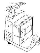
Tow tractors are straight-forward, operator-aboard, self-powered tractors for towing wagons or carts over long distances. Some can operate outdoors.
