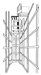
Outrigger rising-cab turret trucks lift the opcrator to the same height as the pallet. These trucks are for stacking pallets on both sides of very narrow aisles to 40-ft heights.
