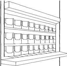
Vertical carousels provide high-density storage. Systems hold small parts or work-inprocess in storage bins on shelves that rotate vertically.
