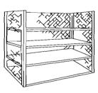
Shelf-type truck superstructures customize a nontilt platform truck to carry loose items and packages and make the truck useful for orderpicking. Counterbalanced lift trucks can be
