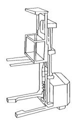
Orderpicker trucks place the operator on an elevating platform along with the forks. The operator picks items or cases from racks onto a pallet or shelf-type structure.
