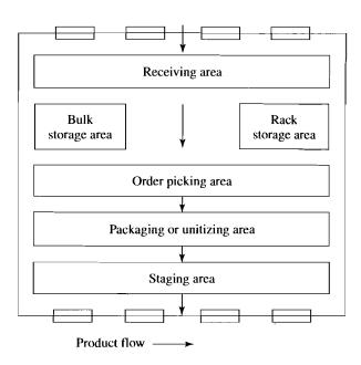
Warehouse design should maximize cubic utilization. Most warehouses are designed with 20- to 30-foot clear ceilings, although modern automated and high-rise facilities effectively use heights over 100 feet. Maximum effective warehouse height is limited by the safe lifting capabilities of materials handling equipment, such as lift trucks, rack design, and fire safety regulations imposed by sprinkler systems.
