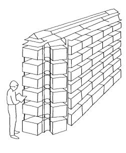
Horizontal carousels store small parts or work-in-process in tote boxes or other containers. Some carousels are self-loading, using automatic equipment for high efficiency.
