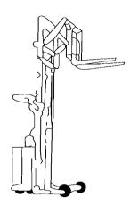
Reach trucks operate in narrow aisles, storing and retrieving pallets in racks. Some are equipped with a pantograph mechanism and can shelve pallets two-deep.
