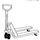
Pallet trucks or "pallet jacks" remain one of the basic unit-load handlers. Load capacities now reach 10,000 lb. Trucks can be customized with options such as skid adapters.
