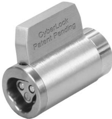
Figure 11-6 In this electronic lock an internal battery moves the cylinder. The key contains embedded data about the key holder, authorization level, and the times and dates of permitted access. ( Photo courtesy of Videx. )
