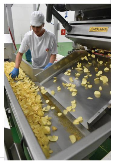
Checking for burned or deformed chips.
