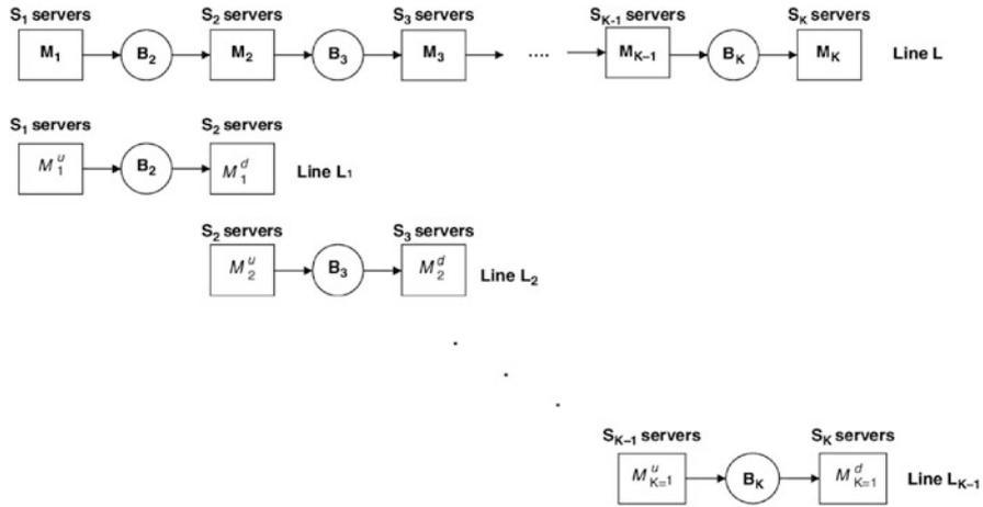
**Fig. 10** Flow line with  $K$  parallel-machine work-stations,  $K-1$  intermediate buffers (Line  $L$ ) and decomposition scheme (Lines  $L_1, \dots, L_{K-1}$ ) (Papadopoulos et al. 2009). In the present work  $S = 1$
