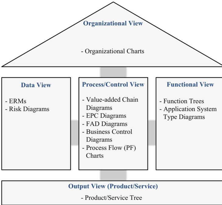
**Fig. 2** Methods of the integrated architecture within different views of “ARIS House”
