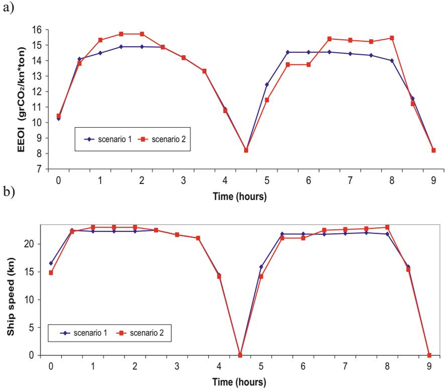
Fig. 4 (a) EEOI time evolution and (b) Ship speed time evolution
