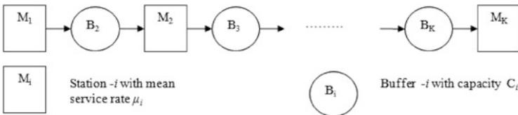
Fig. 7 A  $K$ -station production line with  $K-1$  intermediate buffers
