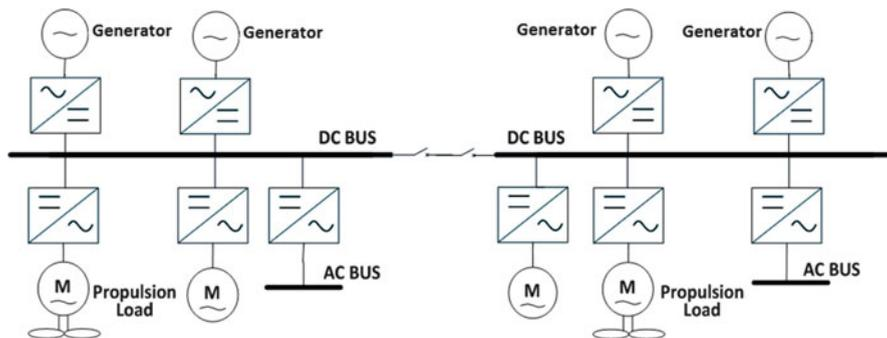
Fig. 1 Generic single-line diagram of AES with dc grid technology
