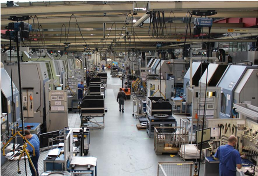
**Fig. 10.4** Machine-centers for turning, milling, and drilling (© Knorr-Bremse Berlin SfS GmbH)
