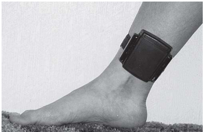
An offender wears an electronic monitoring transmitter. In electronically monitored home detention programs, devices worn by offenders may transmit a signal to inform authorities of the offender's whereabouts. Photo credit: E.S. Boyne.
